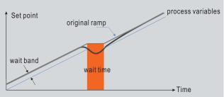
if the process variable is outside the programmed wait band, the ramp in progress will be stopped; it will be restarted when the process variable returns inside the wait band
